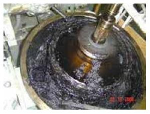
**PRI-STX** prevents severe stability & compatibility problems which can disable purifiers and result in costly vessel delays.
