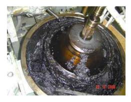
**PRI-SOLV** prevents severe incompatibility problems which can disable purifiers and result in costly vessel delays.
