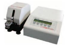
The High Frequency Reciprocating Rig (HFRR) quantifies the extent to which any distillate fuels provide lubricating value
