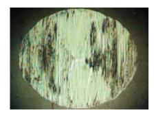
Scar wear in a steel ball subjected to the HFRR test is measured to determine the lubricating property of a given distillate fuel
