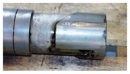
Fuel pump plunger sticking can result from the use of a 0.1% MGO with poor lubricating properties. (Photo courtesy of MAN Diesel)
