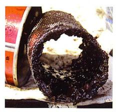
Both heavy fuels and marine gasoils will deteriorate in long-term storage. Pictured is a sludge-plugged fuel filter taken from a diesel standby generator – the result of fuel gone bad.
