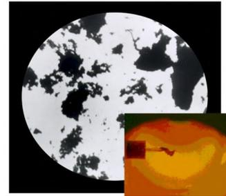
**Untreated Fuel:** High carbon weight structures form during combustion – shown above under an electron microscope and in a burner nozzle test. The result is post-combustion fouling.
