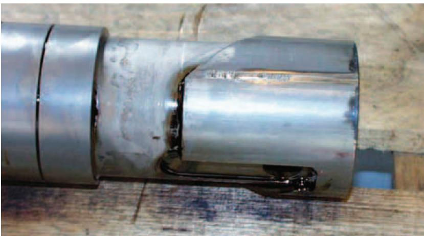
Fuel pump plunger sticking can result from the use of a 0.1% MGO with poor lubricating properties. (Photo courtesy of MAN Diesel)
