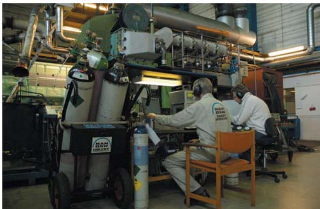
Man B&W technicians monitor emissions testing of a fuel treatment developed by Power Research Inc.
